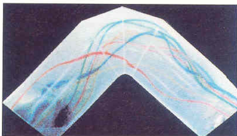
Fig. 2. The CRV pre-rotates the water, imparting a gyroscopic motion to counteract that of the elbow. This produces a uniform flow at the exit of the elbow.
