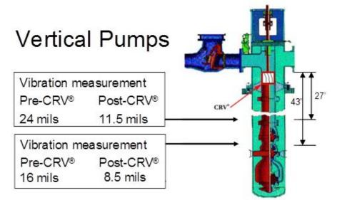
Pre-CRV® installation: Pulsating back pressure, excessive vibration, head box reakage, bearing wear & shaft breakage.
